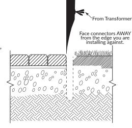
Then, push the EZ Yard Dot all the way into the installation medium. The top of the light will tolerate gentle taps from a rubber mallet if necessary, but never use a metal hammer.
