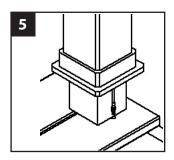
5. Add a small silicone bead around the back of the light.
