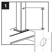
3. Measure and mark the location of the wire pass through hole in the deck board based on the wood post and sleeve. If an aluminum rail is used measure based on the hole in the bottom of the post. use a 3/8" bit to drill the hole for the wire passthrough.
