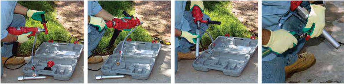
Attach handle; Attach push extension; Attach Diamond Core Bit; Connect to water hose*
