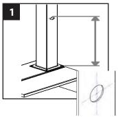
3. Measure and mark the location of the wire pass through hole in the deck board based on the wood post and sleeve. If an aluminum rail is used measure based on the hole in the bottom of the post. use a 1/2" bit to drill the hole for the wire pass through.
