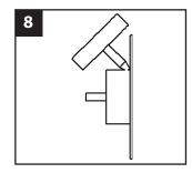
6. Feed wire through deck board. Secure aluminum post to deck board with provided anchor bolts.
